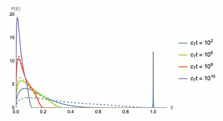
Solid lines: numerical solution starting from  $\delta(E-E_{brk})$ . Dashed lines: attractor solution.
