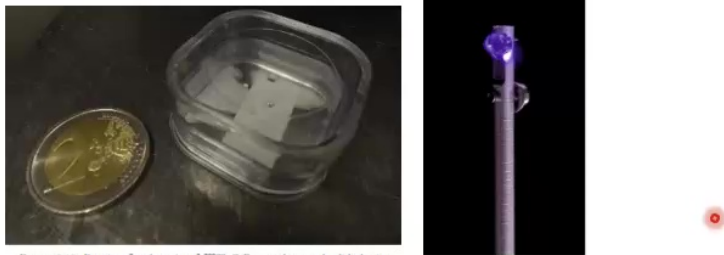
FIGURE 3.18: Four 1 mm 3 and one 4 mm 3 229 Th:CaF 2 crystals cut and polished using above techniques.
