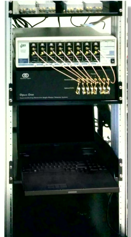
Cryostat and electronics easily rack mountable.
