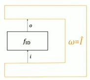
(b) If both f and  $\omega$  are the identity channel, then every possible input is a fixed point. If the input variable i is binary then there are two fixed points (information antinomy).
