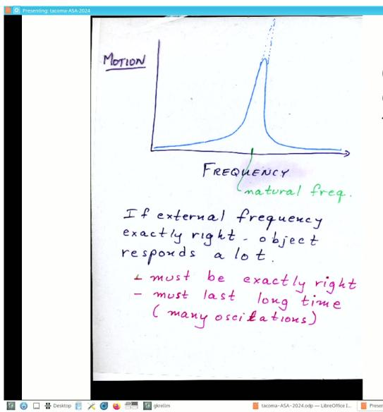
Large response only if driving freq. very close to osc freq. Wind does not behave that way.
