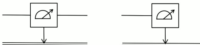
Figure 6: Measurement representation in quantum circuits.
