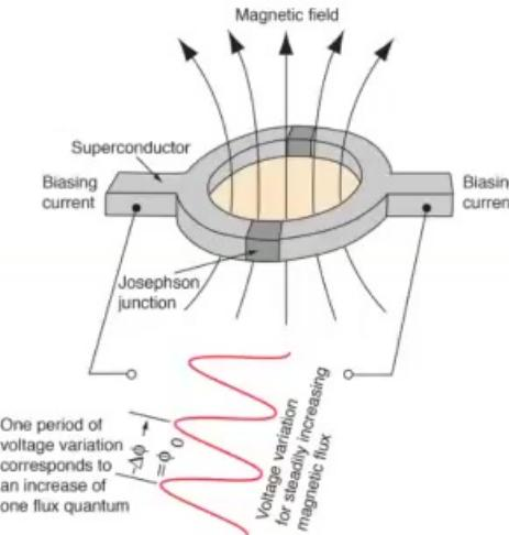
**SQUID: Superconducting QUantum Interference Device** is a magnetometer sensitive to  $\sim 10^{-14}$  T and converts magnetic flux into voltage.
