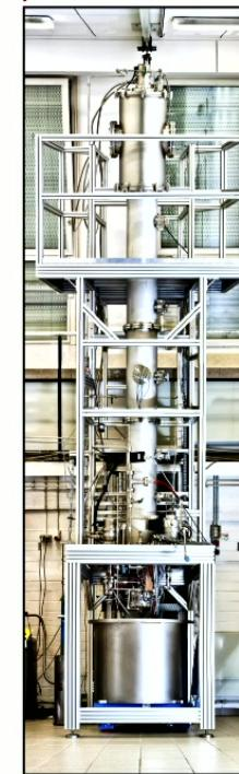
DarkSide Cryogenic distillation column for purification of  $^{39}\text{Ar}$
