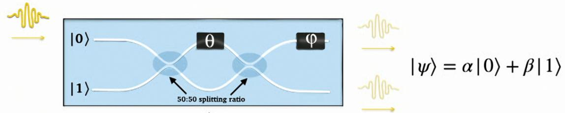
Image of the beam splitter
