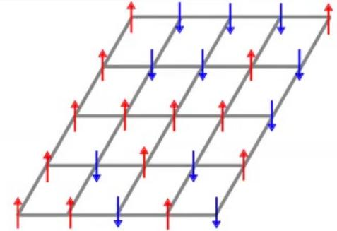
○  $Z = \text{Tr} e^{-\beta E}$  with  $E = -\sum_{\langle ij \rangle} s_i s_j$  ( $s_i = \pm 1$ )
