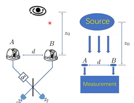
Van Cittert-Zernike theorem: Coherence function g is a Fourier component of the intensity distribution of the sources.
