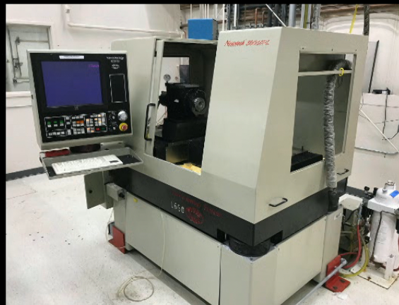
Diamond turning of aluminum mirror at NiPro Optics (not a BREAD part but similar)
