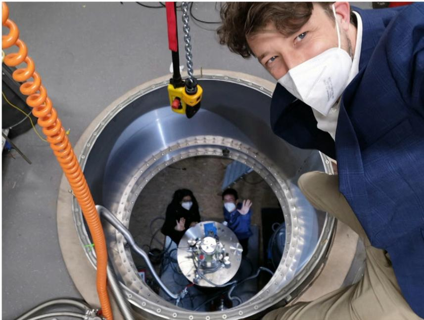
→ liquid  $^{129}\text{Xe}$  NMR apparatus in a high-homogeneity magnet
