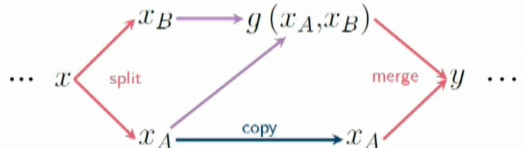
$$\Rightarrow \det \left( \frac{\partial f}{\partial x} \right) = \det \left( \begin{array}{cc} 1 & 0 \\ \frac{\partial y_B}{\partial x_A} & s(x_A) \end{array} \right) = \prod_j s(x_A)_j$$
