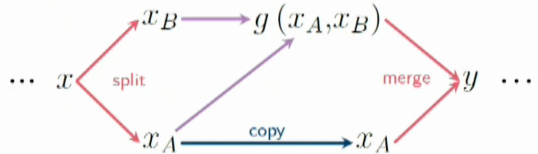
$$\Rightarrow \det \left( \frac{\partial f}{\partial x} \right) = \det \left( \begin{array}{cc} \mathbb{1} & 0 \\ \frac{\partial y_B}{\partial x_A} & s(x_A) \end{array} \right) = \prod_j s(x_A)_j$$
