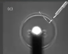
(a) Mach cone near the centre of the jump. (b) Mach cone near the edge of the jump. (c) The Mach cone disappears just outside the jump
