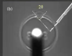
(a) Mach cone near the centre of the jump. (b) Mach cone near the edge of the jump. (c) The Mach cone disappears just outside the jump
