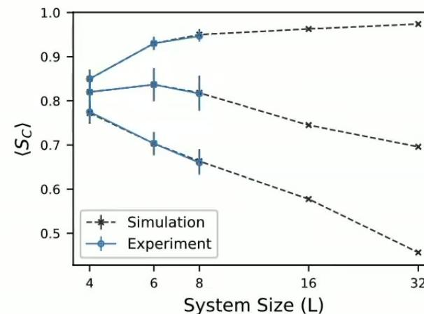
$S_C$  - thresholded entropy after feedback (error mitigation)
