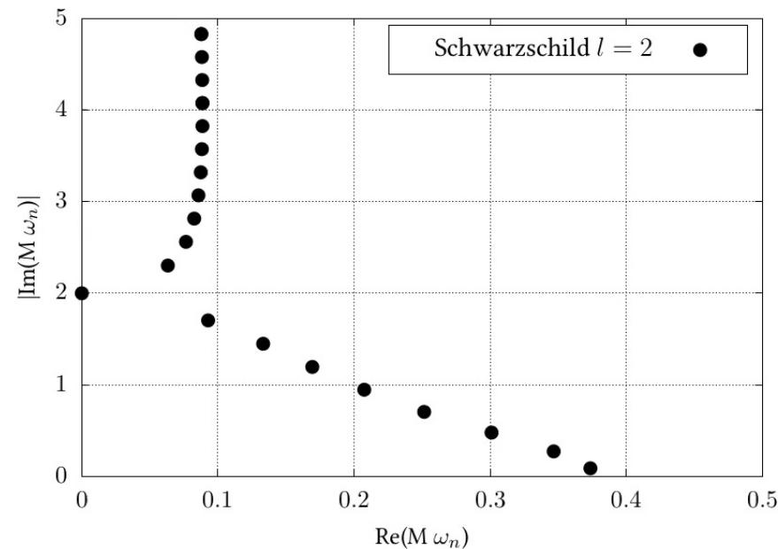
Axial/polar quasi-normal modes on the complex plane for  $l = 2$ . Asymptotic branch continues parallel to  $y$ -axis. Shown spectrum based on Leaver's method.
