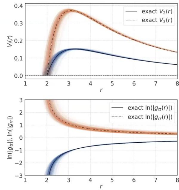
Results for using  $l = 2,3$  and  $n = 0,1$  QNM spectrum with  $\pm 1\%$  relative error. Left: MCMC parameter estimation. Right top: Exact (black lines) and reconstructed (color lines) potentials  $V_2(r)$  and  $V_3(r)$ . Right bottom: Exact (black lines) and reconstructed (color lines) metric functions  $g_{tt}(r)$  and  $g_{rr}(r)$ .
