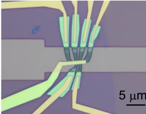
Ferroelectric field effect transistor (FeFET)
