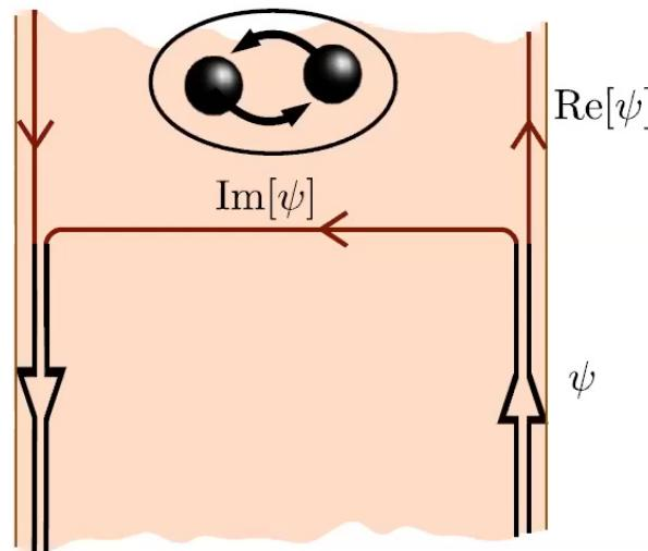
Any charge carrying edge state, fractional or integer, carries an integer thermal conductance  $\kappa_0$
