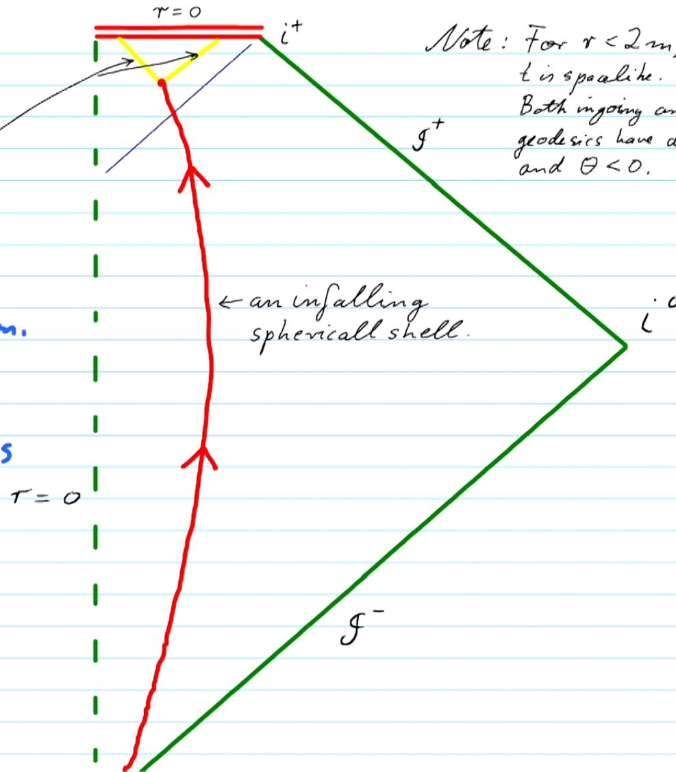
Note: For  $r < 2m$ ,  $r$  is timelike and  $t$  is spacelike. Both ingoing and outgoing null geodesics have decreasing  $r$ , and  $\Theta < 0$ .
