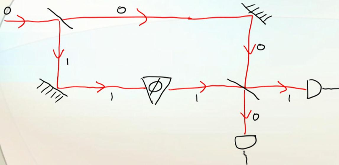
⊙ A general Mach-Zehnder interferometer has 50/50 beamsplitters and a phase shift  $\phi$  on path 1.
