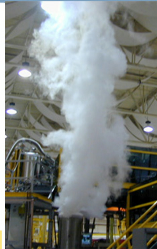
A magnet undergoing a controlled quench.
