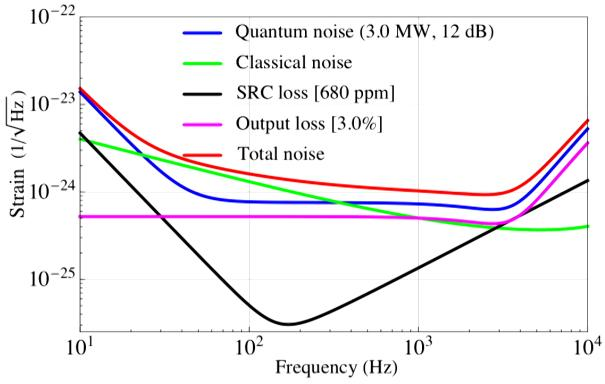
Loss in the signal recycling cavity  $Y_{\text{itmx,y}} = 1000 \text{ ppm} \times \left(\frac{P_{\text{arm}}}{1 \text{ MW}} \frac{\alpha_{x,y}}{0.5 \text{ ppm}} \frac{30}{\kappa_{\text{itm}}}\right)^2$
