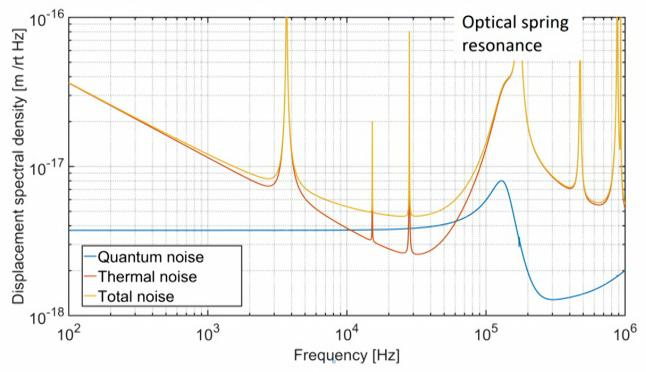
Reshapes noise such that radiation pressure noise is frequency independent below resonance
