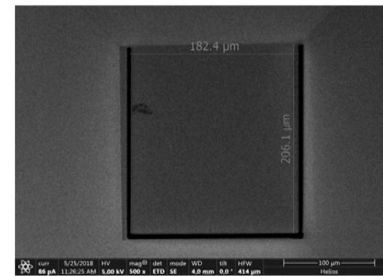
Multiple 6  $\mu\text{m}$  thick AlGaAs/GaAs windows on a 0.5mm think silicon frame
