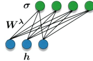
**Restricted Boltzman Machine:**  $p_{\lambda}(\sigma) = \frac{1}{Z_{\lambda}} \sum_h e^{-E_{\lambda}(\sigma, h)}$
