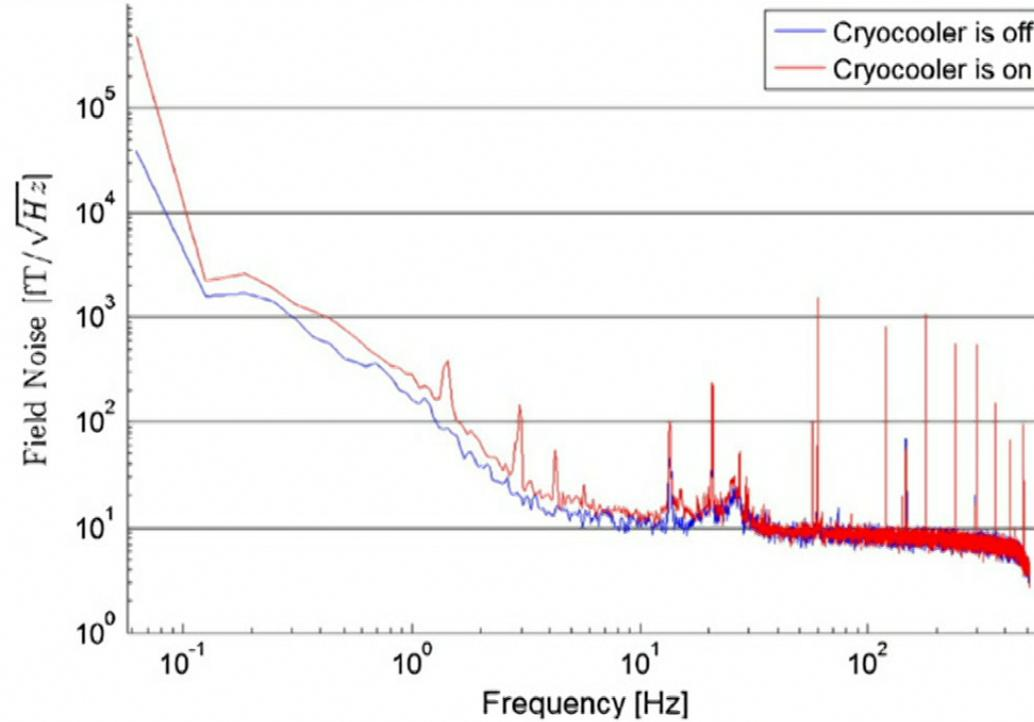
Fig. 8. Raw output of a magnetometer channel in the inner layer of the sensor array with and without the recycler on.
