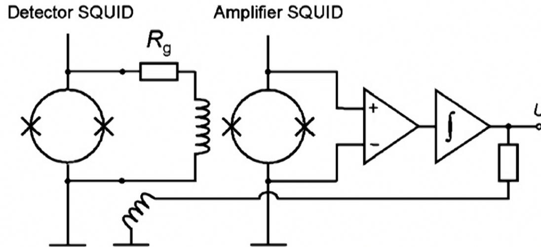
Use a second SQUID as the amplifier of the first (detector) SQUID
