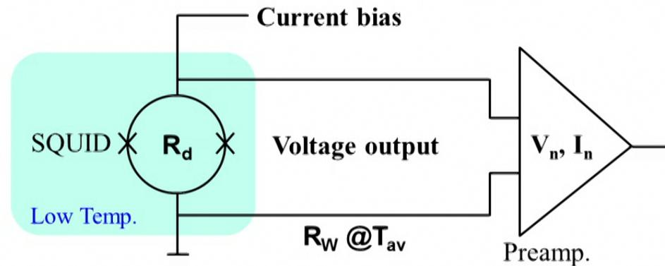
Noise of SQUID system:  $\Phi^2_{\text{intrinsic}} + \Phi^2_{\text{preamp}}$
