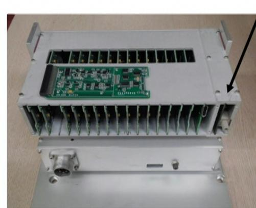
*16-channel electronics for magnetoencephalography*
