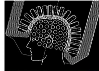
CTF Axial gradiometer (baseline 50 mm)
