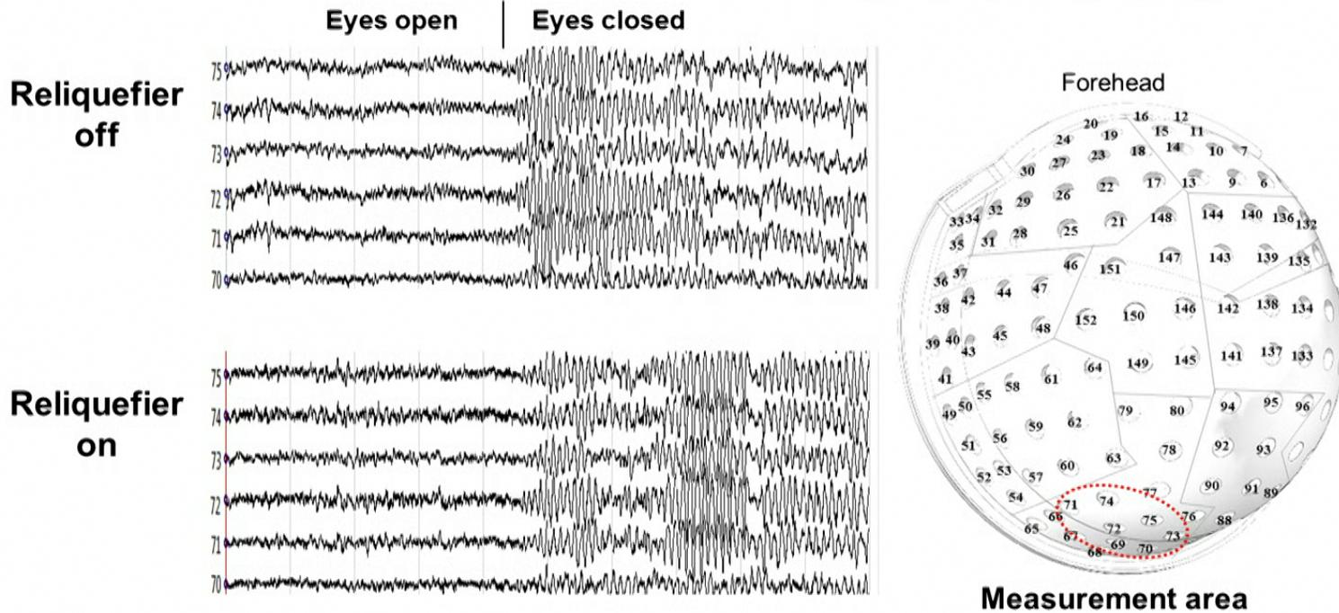
Reliequiefier does not introduce appreciable noise on the brain signal (noise).
