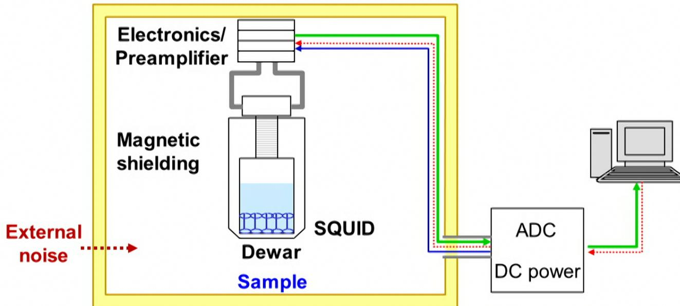
SQUID system noise: SQUID intrinsic noise + Electronics noise
