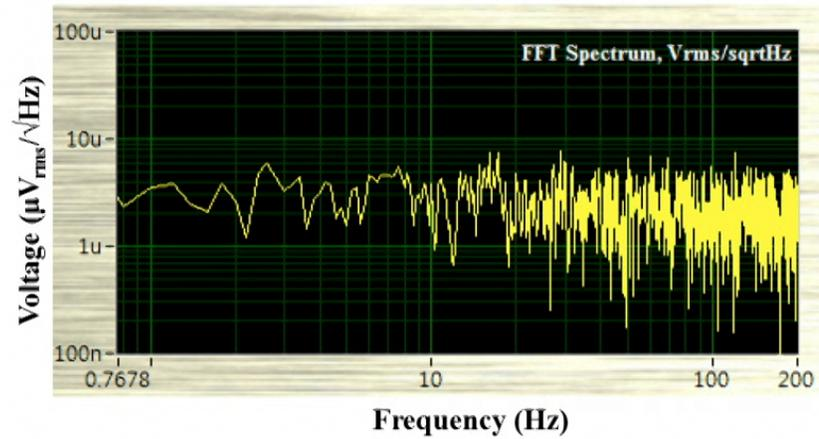
System sensitivity:  $3 \text{ fT}/\sqrt{Hz}$
