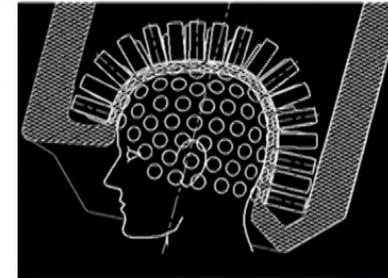
CTF Axial gradiometer
