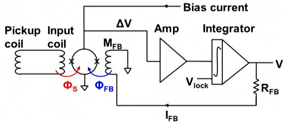
In FLL mode, the flux in the SQUID is kept constant (locked).
