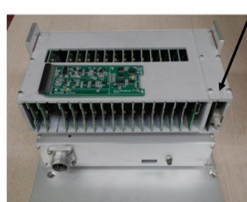
*16-channel electronics for magnetoencephalography*
