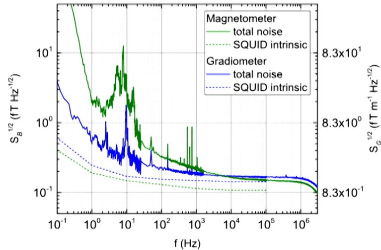
FIG. 2. Measured magnetic flux density noise  $S_{B,m}^{1/2}$  for the two setups with 45 mm diameter pick-up coils: Magnetometer (solid green curve) and gradiometer (solid blue curve). The calculated intrinsic SQUID noise levels  $S_{B,i}^{1/2}$  are given by the dotted curves. For the gradiometer, the noise is referred to the bottom pick-up loop, and the gradient noise is shown on the right.
