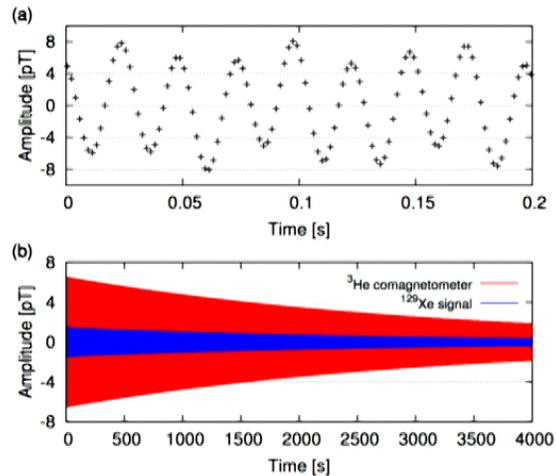
**T2 (transverse spin life-time) are limited by cylindrical cell shape**
