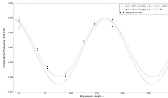
Example: effect of helium magnetization on xenon frequency
