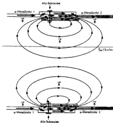
Currently preferred connections of magnetizable materials: 'clamping'
