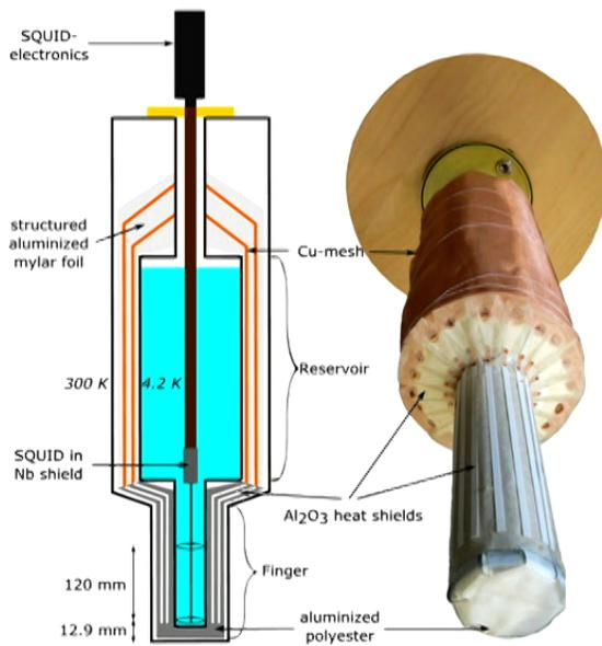
FIG. 1. Left: the schematic setup of LINOD2 in gradiometer configuration. Right: a view of one of the heat shields made from  $\text{Al}_2\text{O}_3$  strips together with the copper mesh heat shield at the dewar reservoir. The outer shell has been removed.
