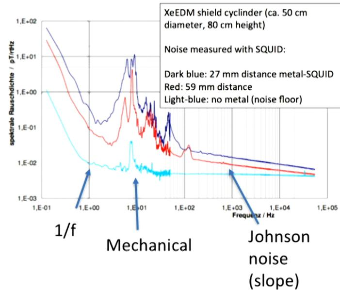
(Measured by PTB, baseline limited by instrument noise)
