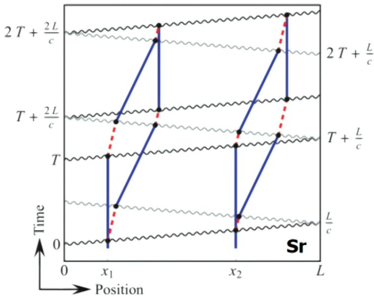
Signal from light propagation time between atom ensembles.
