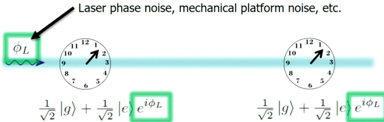
Laser phase is **common** to both atoms – rejected in a differential measurement.
