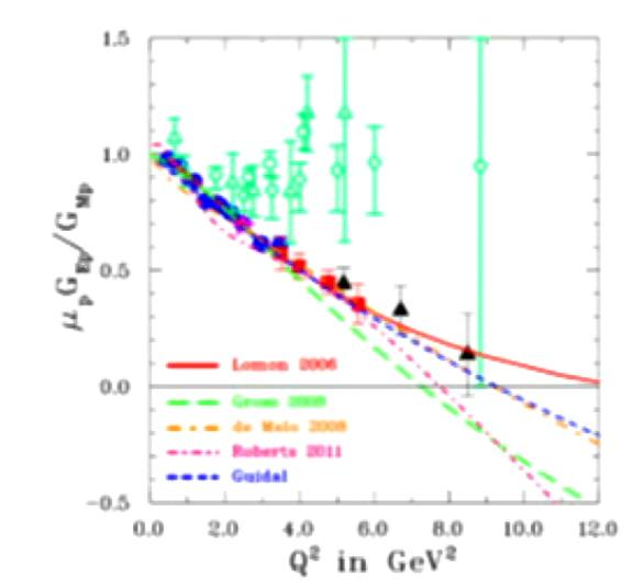
The ratio  $G_{Ep}/G_{Mp}$  obtained by the recoil polarization technique (Punjabi et al. (2005) (filled blue circle), Puckett et al. (2012) (filled red squares) and Puckett et al. (2010) (filled black triangles)) compared to ratio obtained by the Rosenbluth technique (green open points).
