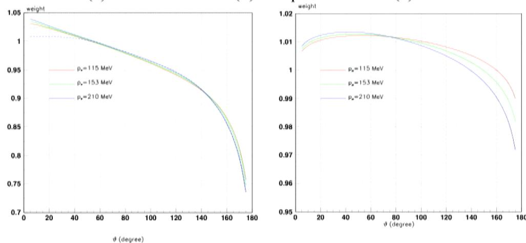
Left: Radiative correction for elastic electron-proton scattering as a function of lab scattering angle in MUSE kinematics. Dashed lines show the effect of a kinematic cut. Right: Same result but for the scattering of muons.
