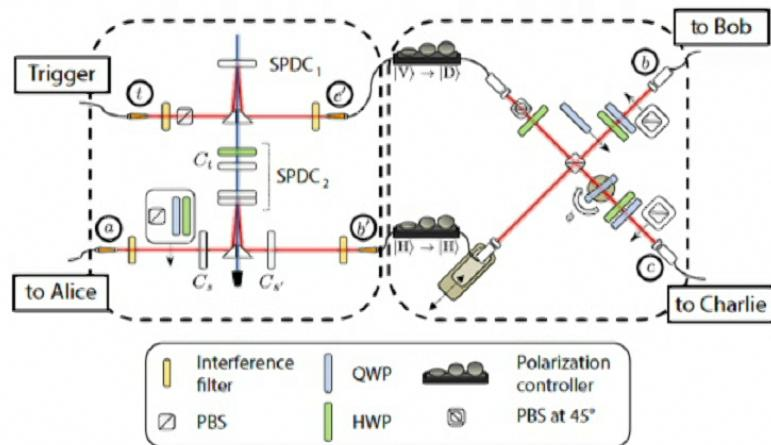
in modes a, b, and c. With no analyzers in place we directly measured the singles rates of 576 kHz, 386 kHz, 417 kHz, and 476 kHz for modes a, b, c, and t respectively, and a four-fold coincidence rate of 39 Hz.
