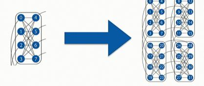
For a quantum annealer with chimera topology the hardware scales linearly in the number of spins
