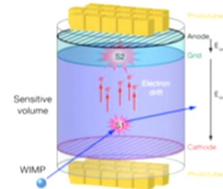
Figure 14. Schematic of a dual-phase LXe TPC
