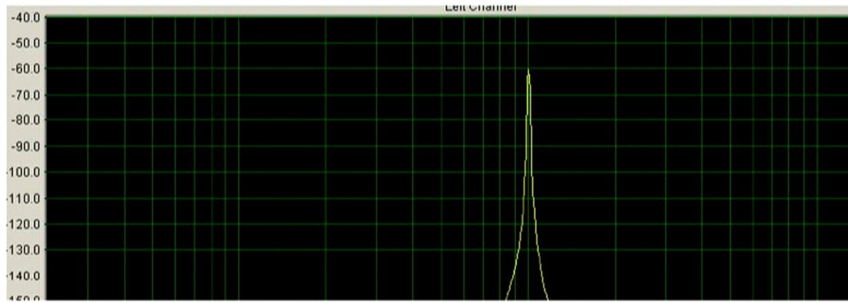
Fourier transform of 1 kHz pure tone recorded at 24 bit depth
