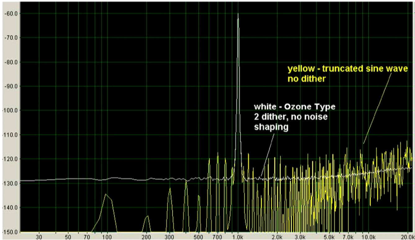
Fourier transform of 16 bit representation of 1 kHz signal,
