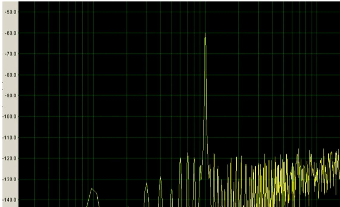
Here's the Fourier transform of the same 1 kHz tone, represented with 16 bits per sample.
