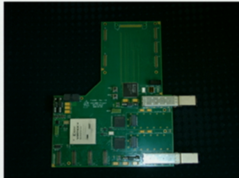
Figure 3 Picture of the FiLa10G board. On the right side the 10 Gbit optical connectors can be seen.
