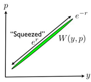
Wigner function is a gaussian with ellipsoid axes
