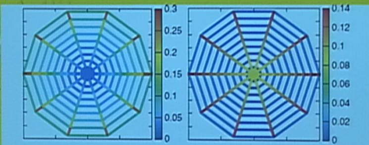
FIG. 2 (color online). Force distribution for undamaged webs (left) for  $K/k = 1$  and (right) for  $K/k = 10$ . The right-hand plot corresponds to natural spider webs. Note that the maxima of the color scale are different in the two plots where the values are given in  $\bar{K}\Delta$ .
