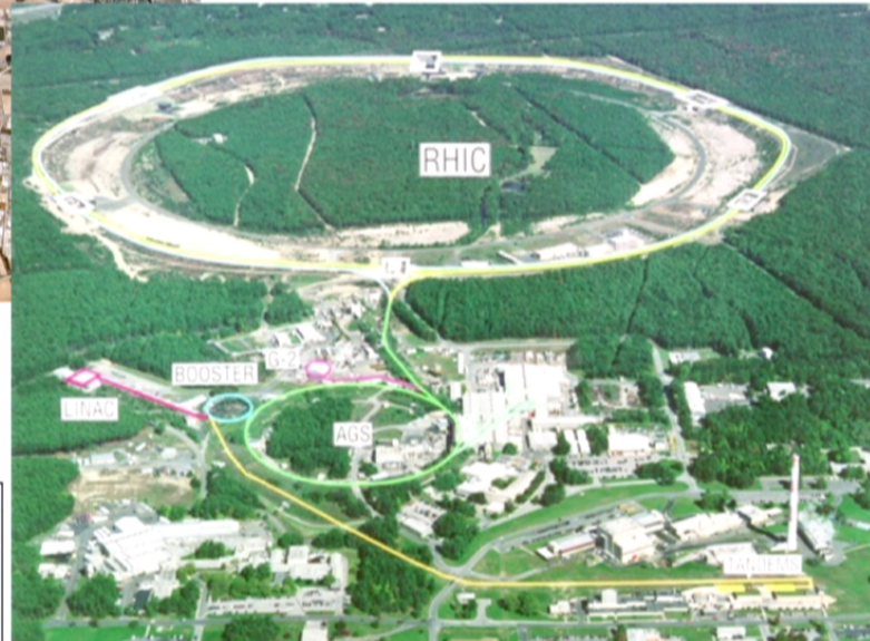
The Relativistic Heavy Ion Collider 3.8 km circumference Top energy: E_{cm} = 200 \text{ GeV/NN}
