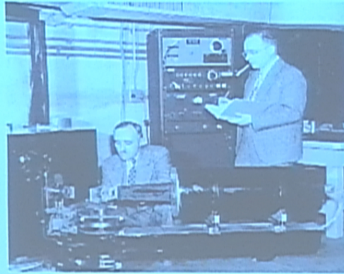
Cliff Shull 1950 confirmed AF ordering in MnO and NiO using neutron scattering 1994 Nobel Prize
