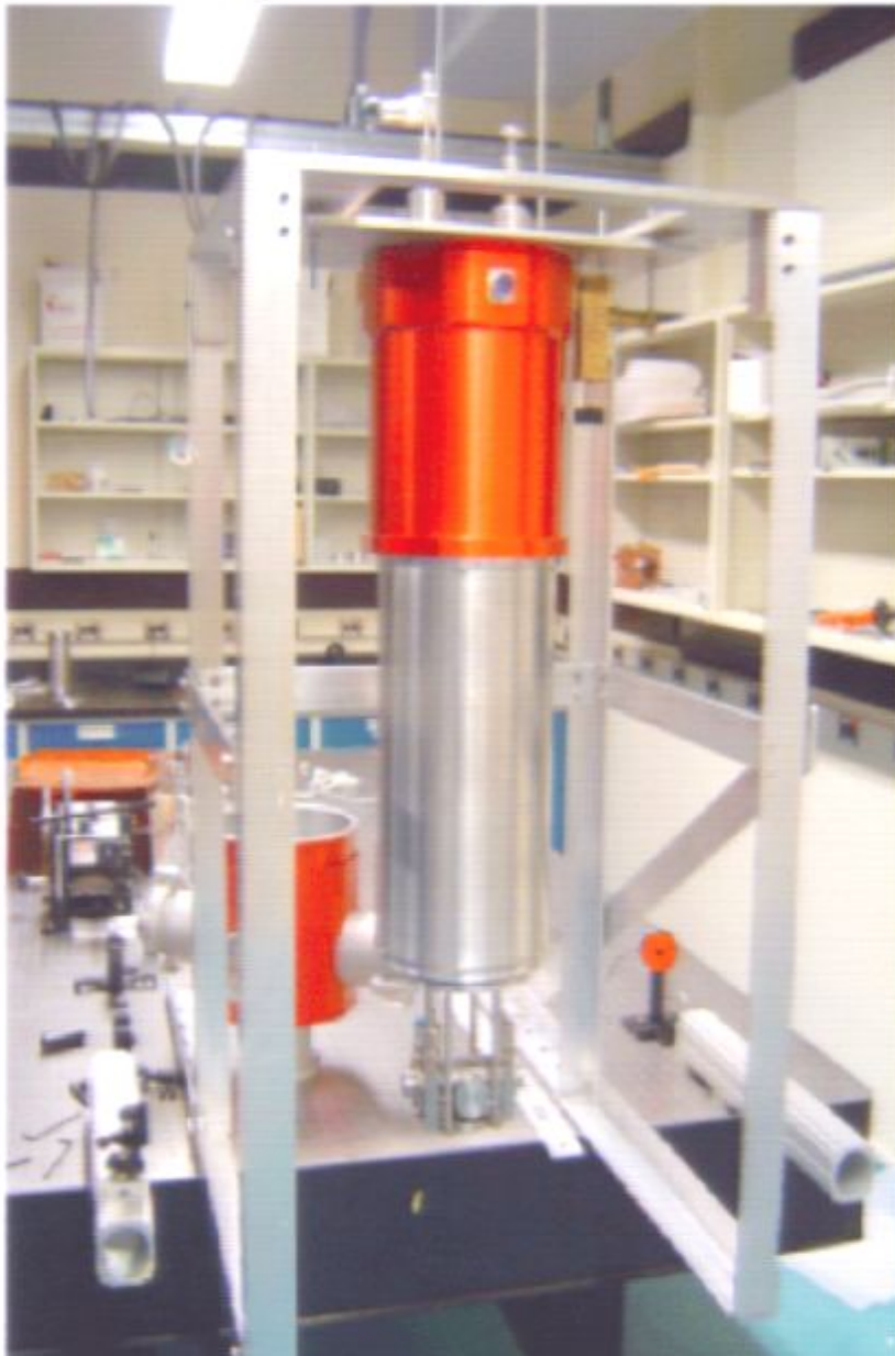
Pumped He-4 system at Yale, with optical access
