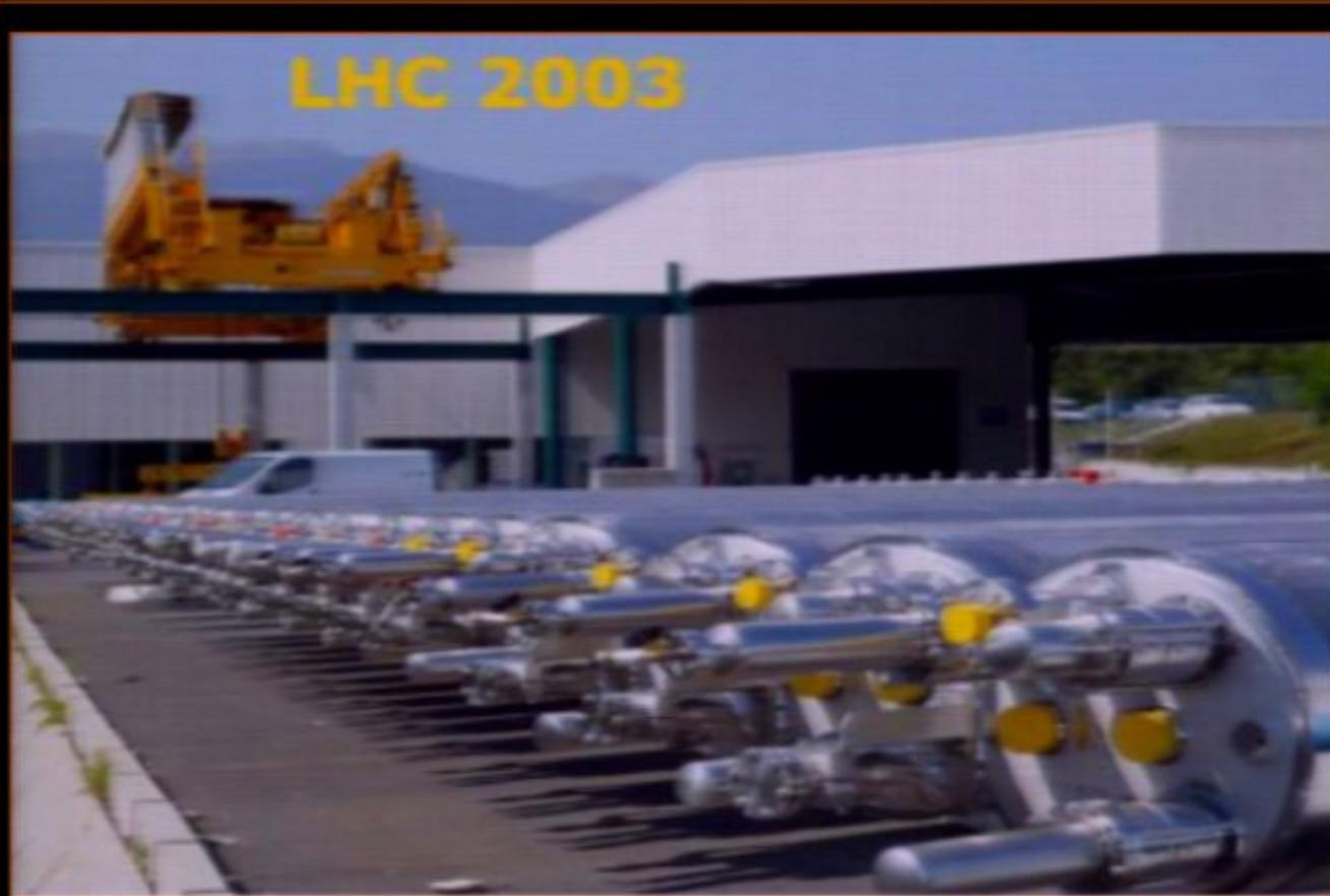
1200 superconducting magnets
