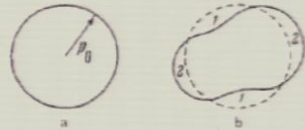
(a) unperturbed distribution (all states inside occupied). (b) perturbed distribution; in regions 1, \delta n = -1 , in regions 2, \delta n = 1 ; inside the solid line all states are occupied.
