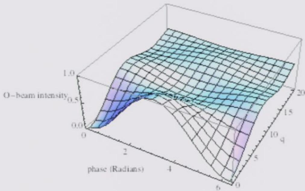
see that as expected all neutrons are detected at one beam or the other, but as the wave-number of the prism is increased the contrast vanishes.
