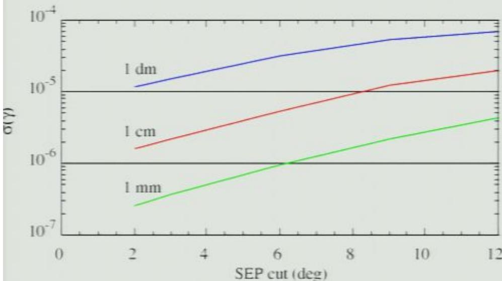
Estimated uncertainty in PPN  $\gamma$  as a function of data accuracy and data cut-off with angular separation from the Sun as viewed from Earth.
