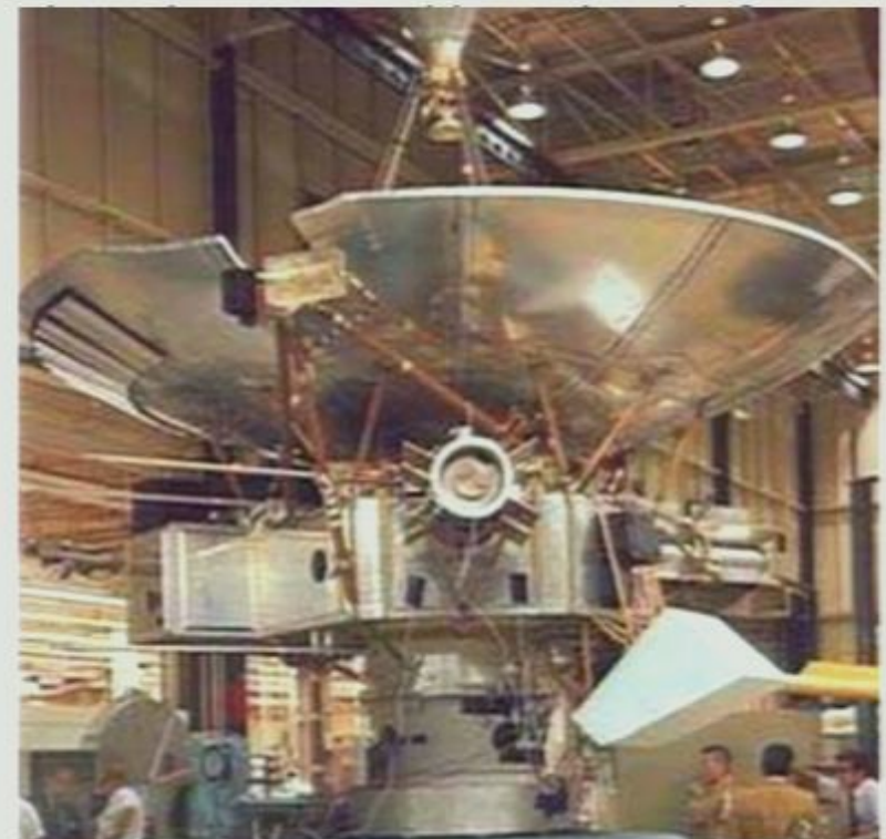
Test Article in Thermal Model Test (Mix of Flight and Non-flight H/W)
