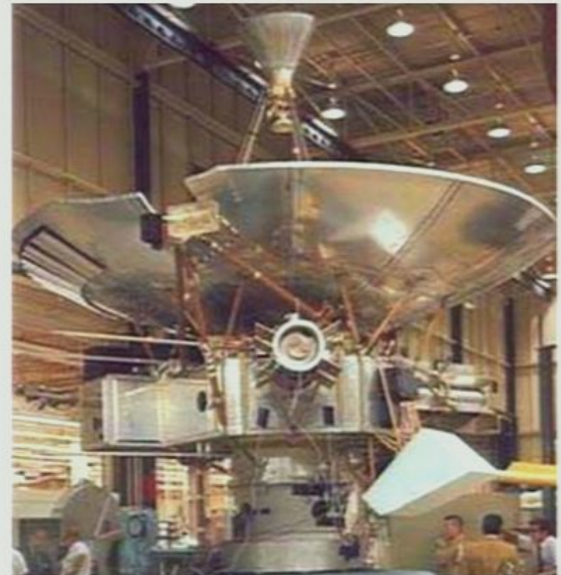
Test Article in Thermal Model Test (Mix of Flight and Non-flight H/W)
