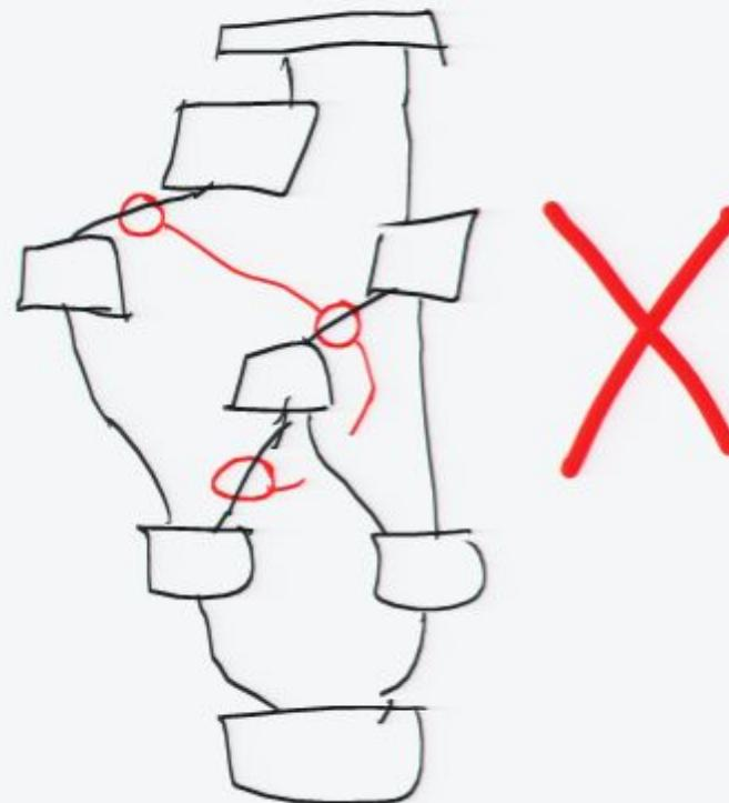
A space-like hypersurface is a synchronous set that partitions the circuit into two parts
