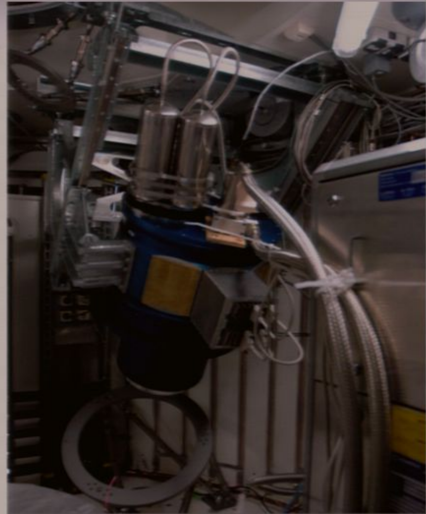
APEX-SZ Camera shown mounted in cabin with pulse tube lines & ballasts visible.
