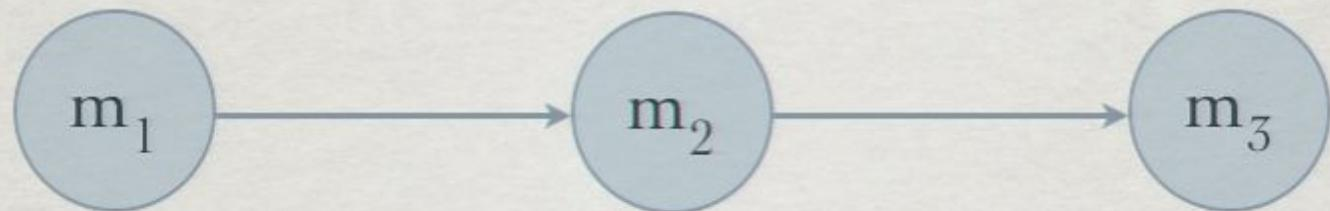
$$\begin{aligned}P(C) &= \Pr(m_2, m_3 \mid m_1) \\&= \Pr(m_2 \mid m_1) \Pr(m_3 \mid m_2, m_1)\end{aligned}$$
