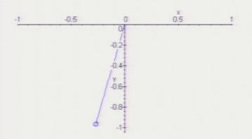
Simple Pendulum in Phase Space: Damped with Coef f= 0.4
