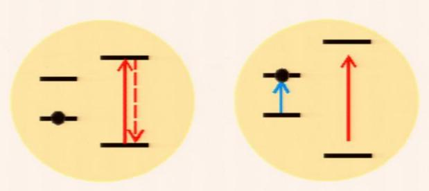
Nucleus in the ground state; laser-induced fluorescence from the shell. Laser excitation of the nucleus; change of hyperfine structure detected in intensity or polarisation of fluorescence.
